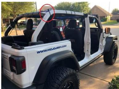
Repeat the process on the other rear corner. (You should now have the front four and the rear two bungee balls attached.)
