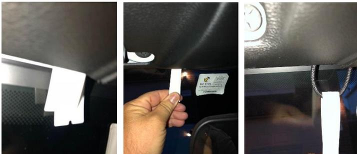
Attach the bungee end to the ball and repeat the same process on the passenger side corner attachment point. (Remember to put the bungee to the outside of the windshield mounting bolt)
