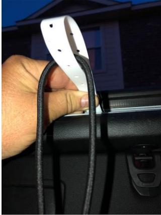
Step 6. Push the plastic tool through the gap between the roll bar and the windshield frame. You will see the pinched ends coming out of the gap next to the glass of the windshield. Pull the plastic tool all the way through the gap.
